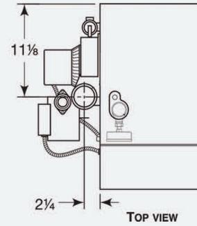
**Note:** Boiler circulator is shipped loose. Circulator may be mounted on either boiler supply or return piping. See dimension chart for pipe size of circulator flange provided.
