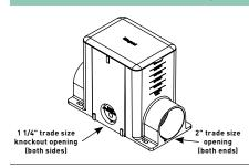
Box comes complete with reusable mudcap, insert spacer, conduit plugs and reducers. Reducers provided for reduction to 1 1/2", 1 1/4", 1", 3/4" and 1/2" [38mm, 32mm, 25mm, 19.1mm and 12.7mm] conduit. Minimum concrete depth is 4" [102mm] and maximum concrete depth is 6" [152mm]. Minimum capacity is 50 cu. in. [819mt] and maximum capacity is 100 cu. in. [1639mt]. Box dimensions are 4 1/8" W x 8 1/4" L x 6 3/16" [105mm x 210mm x 157mm].
