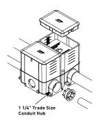
Box comes complete with reusable mudcap, insert spacer, conduit plugs and reducers. Reducers provided for reduction to 1 1/2", 1 1/4", 1", 3/4" and 1/2" [25mm, 19.1mm and 12.7mm] conduit. Minimum concrete depth is 4" [102mm] and maximum concrete depth is 6" [152mm]. Minimum capacity is 50 cu. in. [819mt] and maximum capacity is 100 cu. in. [1693mt]. Box dimensions are 4 1/8" W x 5 1/2" L x 6" H [105mm W x 140mm L x 152mm H].
