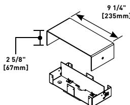
Double width housing for 241 Series Service Head. Barrier included (may not be needed for single service applications). Base has a 3/4" trade size KO for connection to FIT insert. See faceplates on this page. Order two plates to complete service head assembly.
