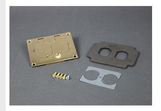
Brass duplex cover plate, 3.156" x 4.182" [80.2mm x 106.2mm]. Flip lids can also be used with 106 type frames for communications. NOTE: Brass covers and flanges are not interchangeable with aluminum or nonmetallic covers and flanges. Nonmetallic covers are interchangeable with aluminum flanges.
