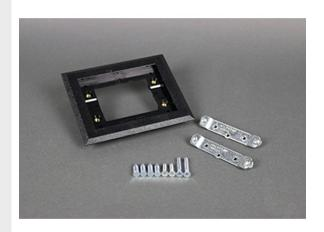
One-gang nonmetallic carpet flange. For Ortronics connectivity use with 829PFLRT Cover. For Wiremold Open System connectivity use with 829PFL Cover. Accepts Ortronics® MAB6TJ TracJack, MAB3S2 Series II and Wiremold CM Series Open System adapters, sold separately. NOTE: Polycarbonate cover plates can only be used with polycarbonate flanges.
