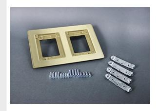
Two-gang brass combination carpet and tile flange, 6.080" x 9.185" [154.4mm x 233.3mm]. Accepts Ortronics MAB6TJ TracJack and MAB3S2 Series II, and Wiremold CM Series Open System adapters, sold separately. NOTE: Brass cover plates can only be used with brass flanges. Brushed aluminum flanges come with beveled edges.
