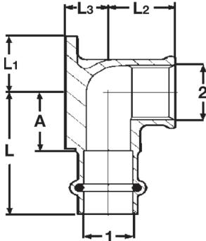
Bronze Elbow Drop 90° P x FPT with Wall Plate - Model 2925.5ZL
