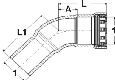
Viega MegaPress 45° Elbow, Carbon Steel, FTG x P - Models 4826.1 / 6626.1
