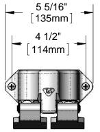
3 9/16" [90mm] Closed 2 7/16" 25mm 61mm 2 9/16" 2 1/4" 1 15/16" [65mm] 57mm [49mm] 4 1/4" 1/2" NPT [109mm] Female Closed Inlet 1/2" NPT Female 4 5/16" Outlet [109mm] Knee Pedals Hang Outside of Cabinetry for Knee Access
