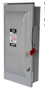
Siemens Low Voltage Circuit Protection General Duty Safety Switches. Type: Safety Switch, Enclosed General Duty Special Features: Non Fusible Application: Construction, Industrial, Residential Std: UL98 V. Rating: 240V A. Rating: 100A No. Of Poles: 3 Action: Single Throw Material: Galvanized Steel Size: H 23.46 x W 11.67 x D 14.68 inches Enclosure: Type 3R Mounting: 2 or 3 Point Mounting Lever O. Cycles: UL 98 Cycles Environmental Conditions: Seismic T58569.01-1
