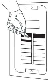
8. Install panel label and Building Occupant's Test Reminder card supplied with the circuit breaker.
