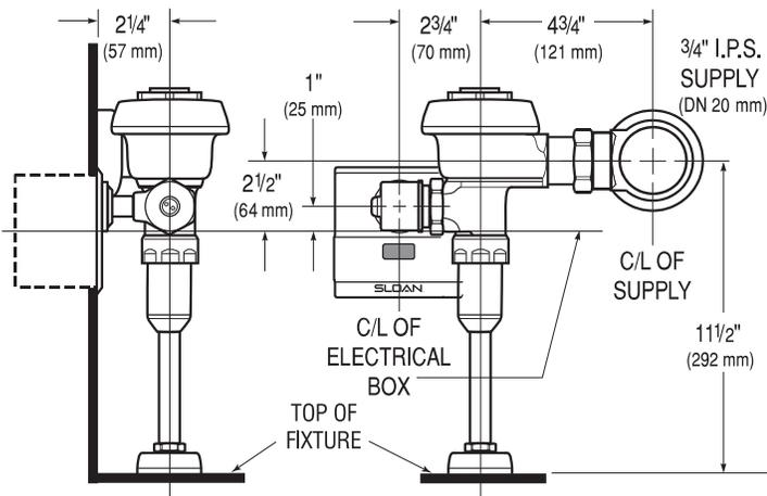
To ensure a perfect rough-in, Sloan recommends the use of the EL-518-A Flushometer Electrical Box Positioning and Support Kit. Specify and order the EL-518-A Kit separately. Consult factory for installation details.
