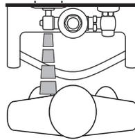
3. When the user steps away from the OPTIMA Sensor, the circuit immediately initiates an electrical "one-time" signal that operates the Solenoid. This initiates the flushing cycle to flush the fixture. The Circuit then automatically resets and is ready for the next user.
