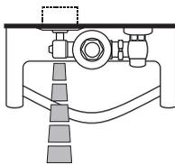
2. As the user enters the beam's effective range (15" to 30") the beam is reflected into the OPTIMA Scanner Window and transformed into a low voltage electrical circuit. Once activated, the Output Circuit continues in a "hold" mode for as long as the user remains within the effective range of the Sensor.
