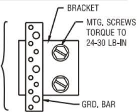
APPROXIMATE LOCATION\* OF EQPT. GROUND BAR MTG. HOLES (2" CENTERS) WITHIN ENCLOSURE.
