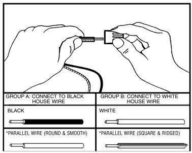
\*Note: When parallel wire is used, the tracer wire is square shaped or ridged and less tracer wire is round in shape or smooth. (Seen best when viewed from wire end.) To separate wires, grasp the ends of each wire and pull apart.
