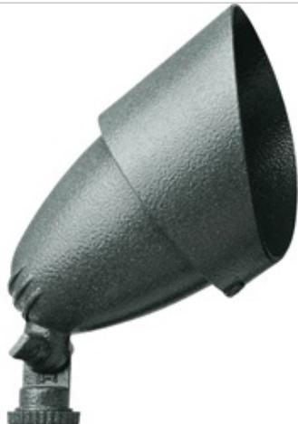
75 Watt Quartz Bullet Flood with silicone O-ring gasket, thick tempered glass lens, internal and external cooling fins. Gold plated socket contacts and 250°C Teflon coated wires for extended lamp life. Lamp supplied.
