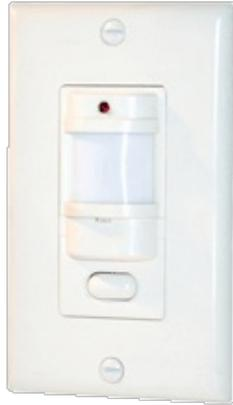
Fits decorator wall plates with only 1/2" protrusion. 120 volts. Gangable. Full 180° view covers 1000 sq. ft Works with electronic ballasts. Can be wired in parallel. LED indicator, wallplate included. Can also be used as a ceiling sensor. Must have hot and wires in box.
