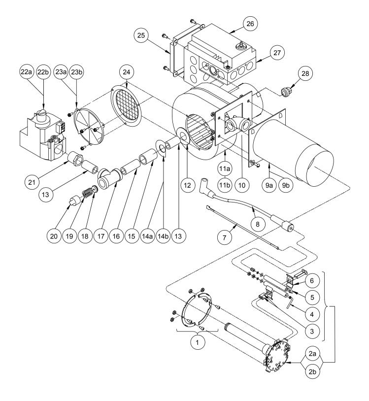
Figure 9: Isometric View of EC200 and EC300
