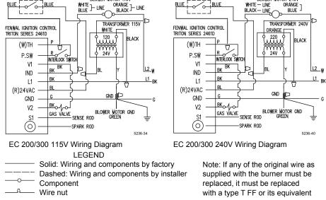
Figure 5: Wiring Diagram
