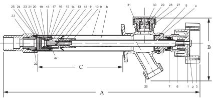
WARING: Hose must be removed in order to prevent freezing or warranty will be null & void!
