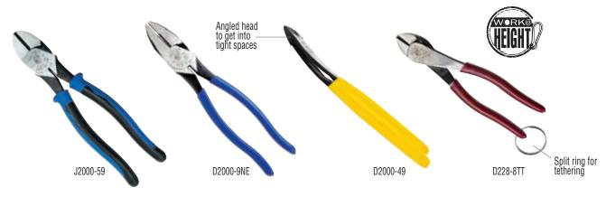
Available in side or diagonal-cutting models, these pliers feature a high-leverage design. The rivet is closer to the cutting edge for greater cutting and gripping power than other plier designs. The 2000 Series have heavy-duty cutting knives for ACSR, screws, nails and most hardened wire. The angled head on the diagonal cutters easily gets into tight spaces. The "TT" series feature a split ring for tethering the pliers when working at height.
