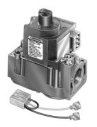
These universal electronic ignition gas controls are used in gasfired appliances with capacities up to 150 cu ft/hour at 1 inch wc pressure drop (4.2 cu m/hour at 0.25 kPa) for natural gas. The VR8245M will operate with a direct spark (DSI), hot surface (HSI) or intermittent pilot ignition. The control includes a manual valve, two automatic operators, a pressure regulator, pilot adjustment, pilot plug and ignition adapter.
