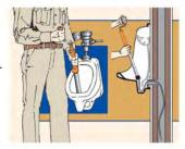
48" spring for clearing stoppages beyond the urinal. TU4 has rust resistant steel tube and rubber bumper to protect urinal bowls.
