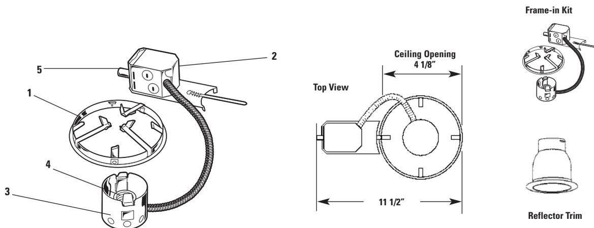
Complete Fixture consists of Reflector Trim & Frame-In Kit. Select each separately.
