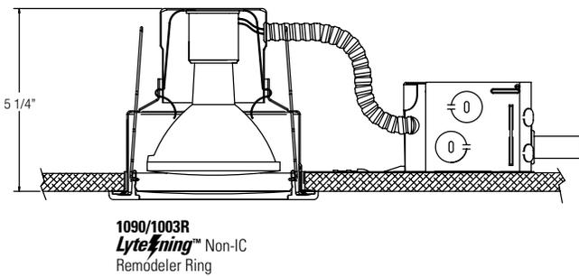
Complete Fixture consists of Reflector Trim & Frame-In Kit. Select each separately.
