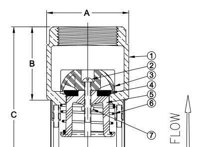
Open Area: 35-50% Max Temp 180°F (82°C) Max Pressure 250psi (18bar)
