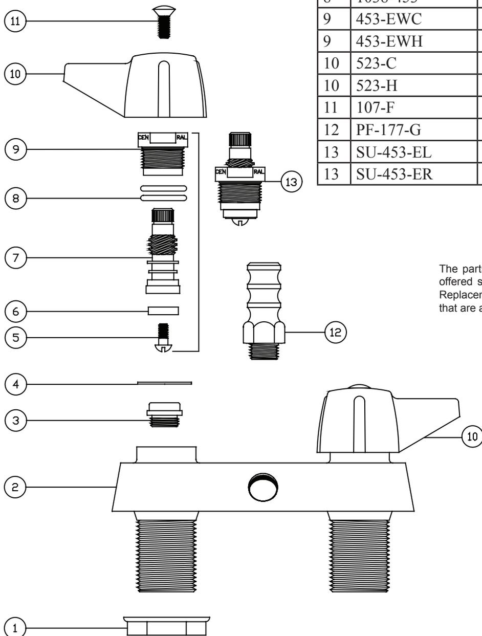
The parts listed in the parts breakdown above may not be offered separately as replacement parts. Please review the Replacement Parts page for the authorized replacement parts that are available for this item.
