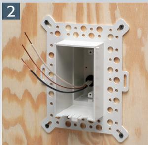
2 Install NM cable connector and wire. Attach recessed IN BOX to substrate, then install moisture barrier around box as shown above in Method 1.
